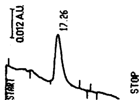
Fig. 3. High-performance ion-exchange chromatography of glucose oxidase on DEAHAP-agarose. Sample, active fraction (main peak) from the experiment in Fig. 1. Column dimensions, 5.6 \times 0.6 cm I.D.; buffer, 0.03 M Tris-HCl (pH 7.6); bead diameter, 5\text{--}10 \mu\text{m} ; elution with a 30-min gradient from 0 to 0.3 M sodium acetate; flow-rate, 0.2 ml \text{min}^{-1} . The figure 17.26 in the chromatogram refers to the elution time in minutes.
